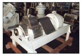
swiveling hammers. This type of grinder is the preferred type when processing whole leaf aloe. The intention of this process is to extract the liquid contained in the aloe leaf. Typically the tips and tails are removed before this step. The particle size is controlled by the size of a mesh placed at the bottom of the grinder
