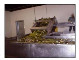
**c.** Manual brushing: Here leaves are hand picked and brushed as they are pulled out of the soaking tank, then they are placed into a conveyor. The advantage of this type of treatment is that it is very gentle on the leaves, and removal of dirt and foreign material is optimal. Also, this can work as an inspection/rejection point. The downside is the higher labor cost.
