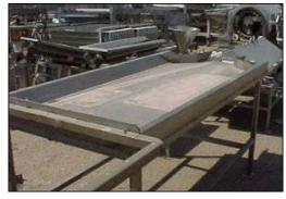
It is important at this step to reject any leaves with evident injuries, cuts, or lesions in order to avoid contamination of the product downstream. Tips, tails, and spines are usually cut off the leaves by hand at this stage, so again the layout is such that would accommodate enough people to perform these duties. Typically 6 to 8 people can process 1000 Kg of leaves through this step.
